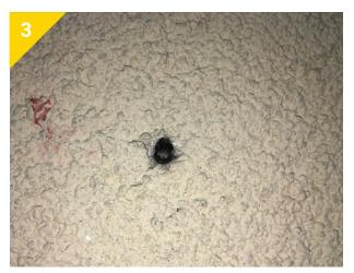
3. Sto IMPACT system not completely penetrated after 54,900 cycles.
