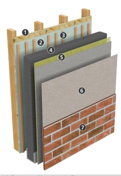
1) Substrate (by others): Glass mat gypsum sheathing in compliance with ASTM C1177, code compliant OSB or plywood sheathing, concrete or concrete masonry, existing structurally sound, uncoated brick or other masonry wall construction.
