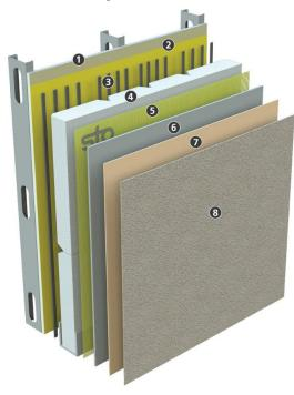
1) Substrate (by others): Glass mat gypsum sheathing in compliance with ASTM C 1177, code compliant OSB or plywood sheathing, concrete or concrete masonry, existing strucuturally sound, uncoated brick or other masonry wall construction.
