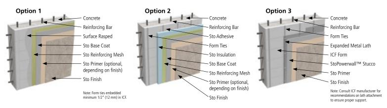
Option 1: Coating System Recommended when the walls are straight and flat with little leveling needed and ties are embedded at least 1/2 inch inside the ICF form.
