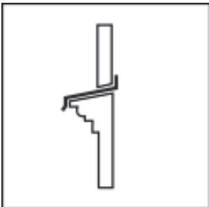
D 4. Provide flashing over build-outs
